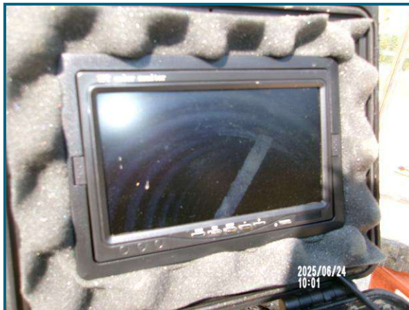
P28. Nail Inside Drain Line
